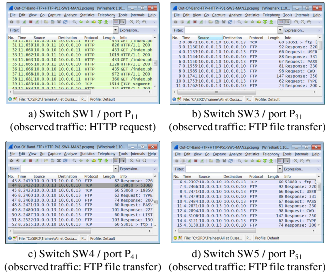
Fig.4. Wireshark traffic captures. The non sensitive HTTP request crosses SW2-SW1-SW5 (SW1 being un-trusted); while the FTP transfer of the sensitive data crosses SW2-SW3-SW4-SW5 (trusted path)
